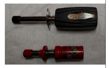
It uses a 1S 1200mAh Li-Po battery, regulated to 1.5V output. It comes with its own dedicated charger and at \$27 is about the same as a comparable conventional glow driver & charger. It is available from Horizon Hobbys.
