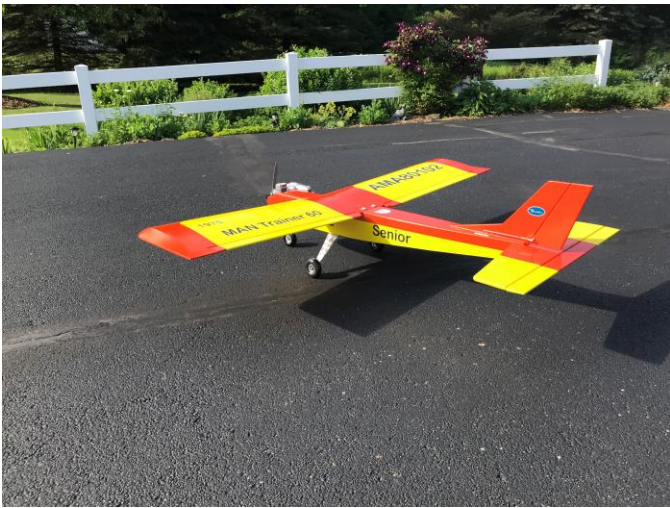
Ray Phillips' MAN Trainer 60 Senior is now ready to fly. Short kit from BalsaWorkBench.com, OS 55 Glow Powered, Spektrum Radio, Hitec Servos and SIG Koverall / Silkspan dope finish.
