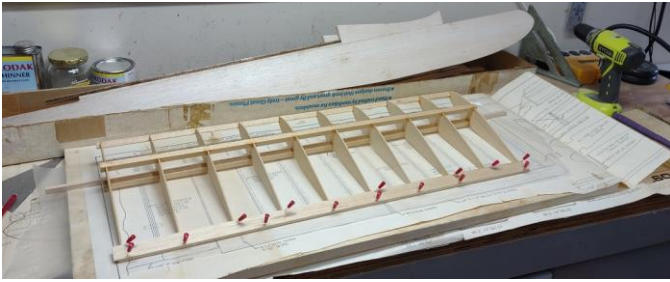
Scott Wallace's RCM Trainer 60 being framed up, aiming to build this with capability for wheels, floats, and skis. Will use a Saito 4 stroke.
