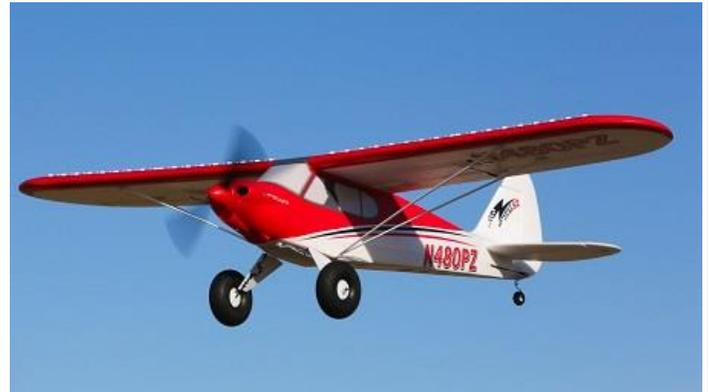
The motor is a 480-size, 960Kv BL out runner. The battery is 3S 1300-2200mAh Li-Po. Since this is a very popular plane a lot has been posted on various web sites about upgrades. There are some good suggestions there but don't plan to upgrade to a different size motor or larger battery system. The whole idea is to race a very affordable plane that is extremely easy to fly.
