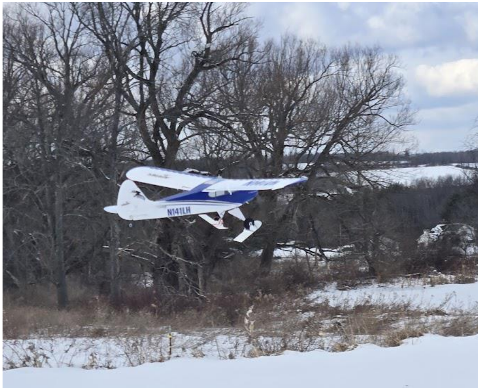
Fig 1-1: The Sport Cub S2 With 3D Printed Skis
